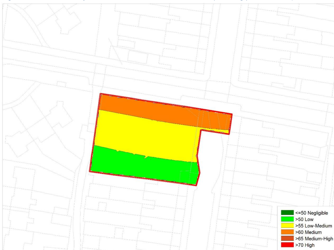
Figure 5-1: ProPG Daytime Noise Contour Plot dB L Aeq,16h (1.5m agl) – Undeveloped
