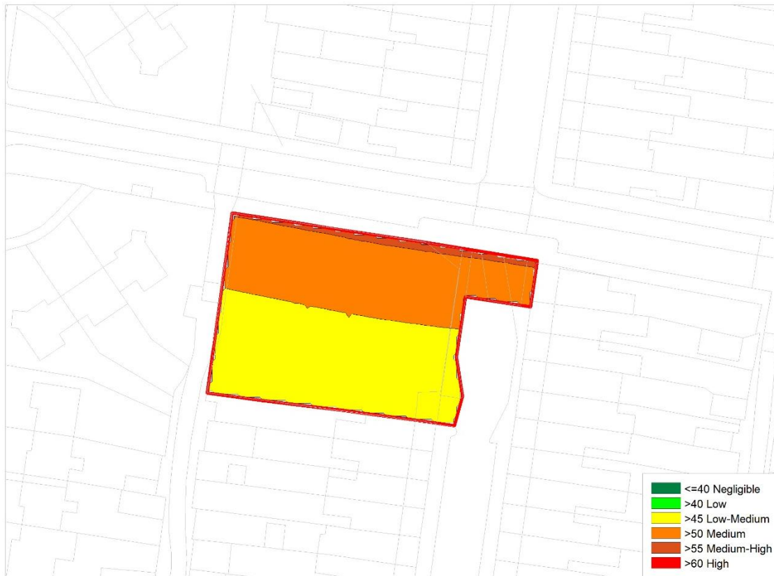
Figure 5-2: ProPG Night-Time Noise Contour Plot dB L Aeq,8h (4.0m agl) – Undeveloped
