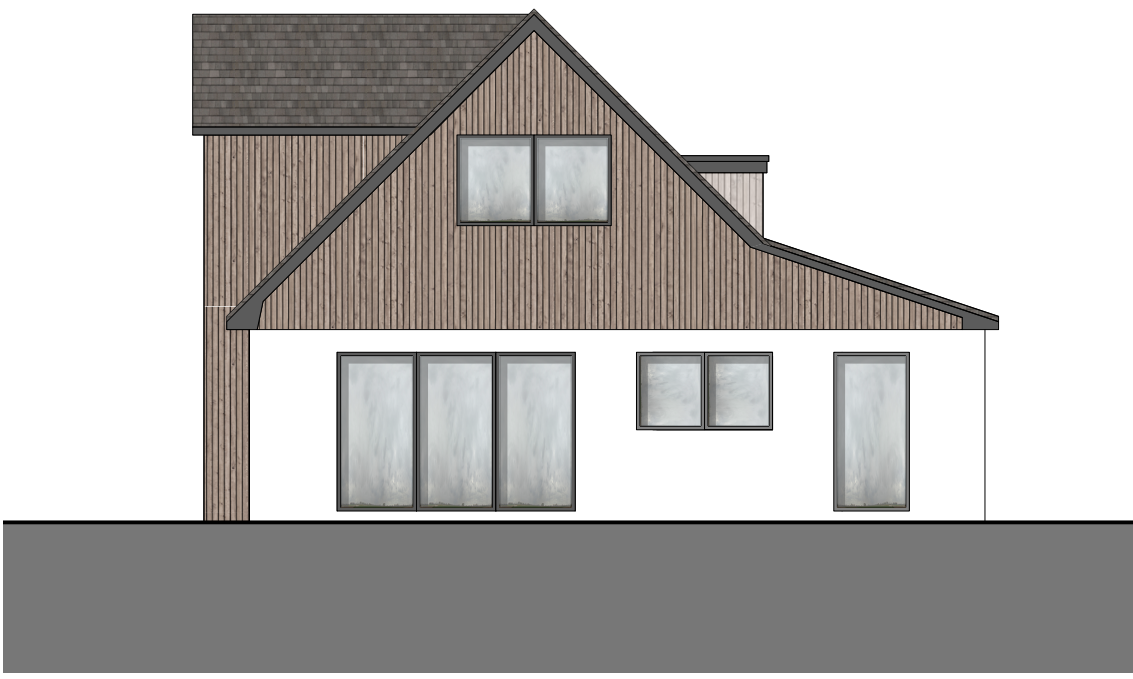
PROPOSED REAR ELEVATION 1:100
