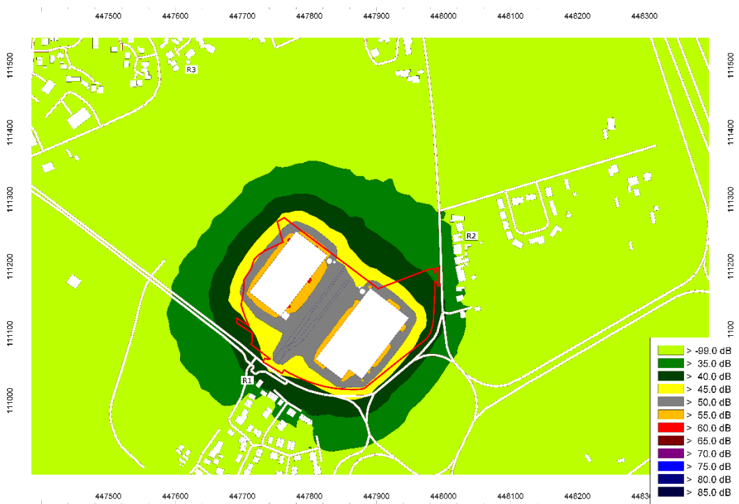
Figure 7.2: Predicted operational noise levels during the night-time (23:00 - 07:00) at a height of 4m (first floor level)
