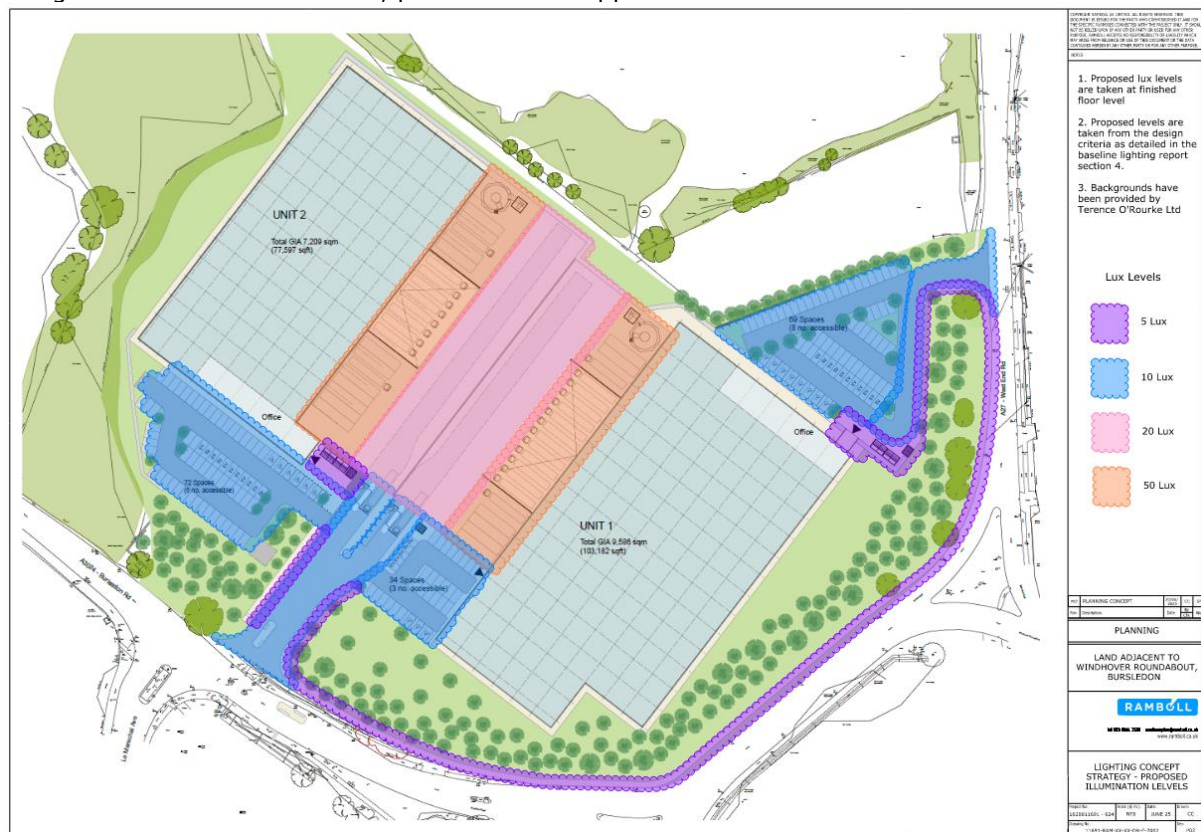
Figure 4. 5: Overall Proposed Illumination Levels
