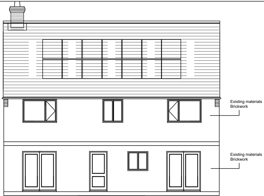
EXISTING REAR ELEVATION 1:100
