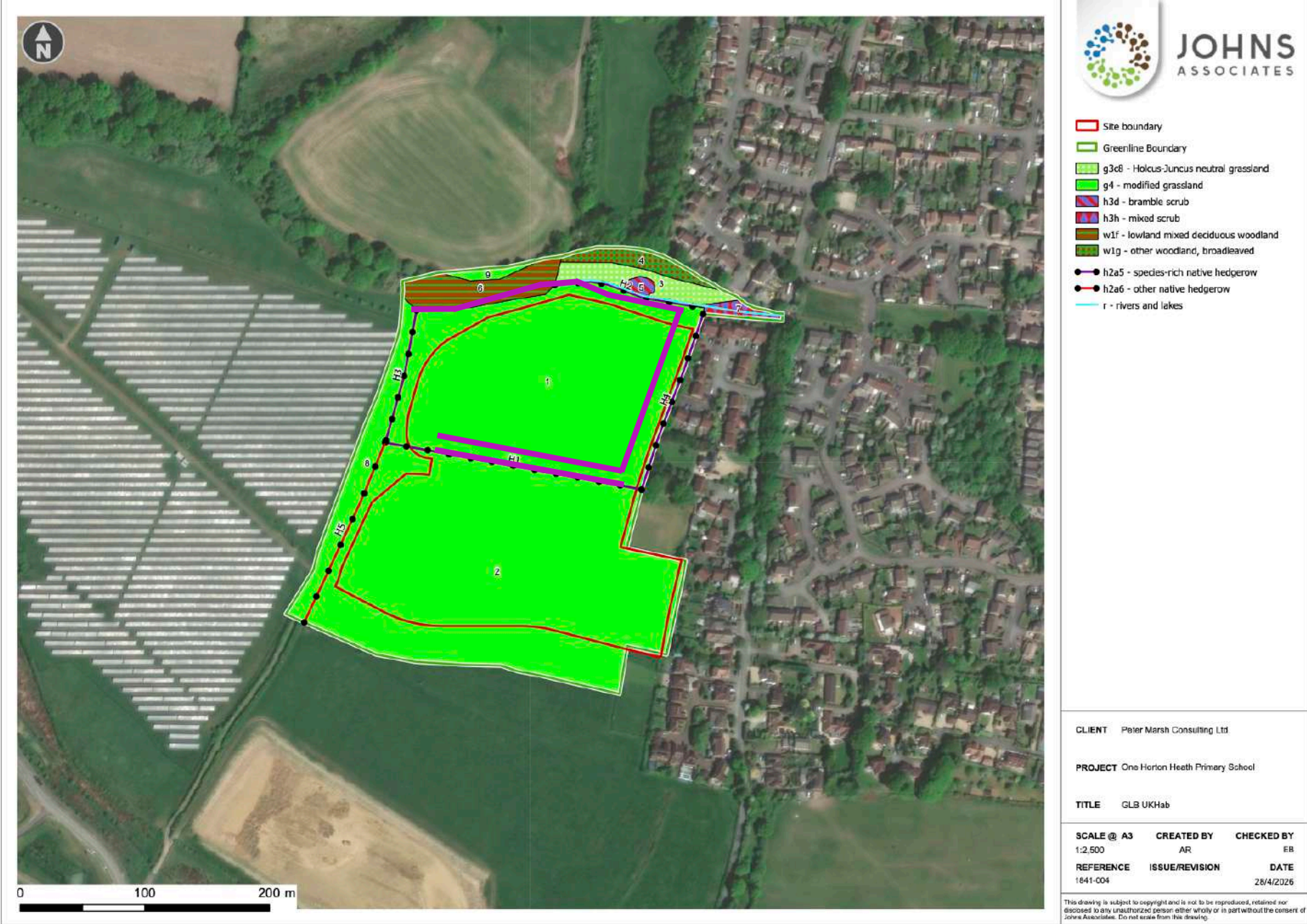
Figure 5: Extent and location of the boundary protective fencing (purple)
