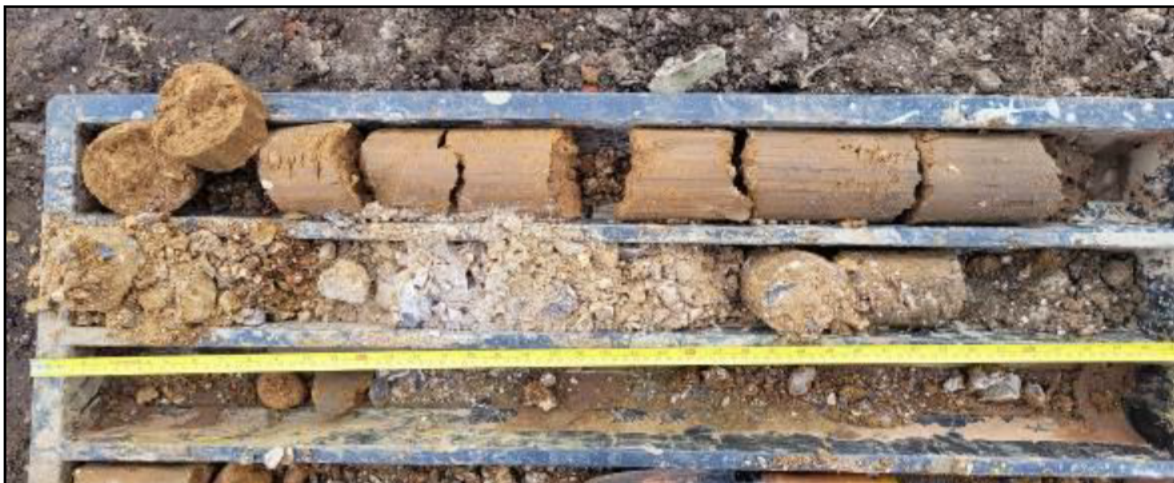
Photograph 2 Removed soil material - BH.02
