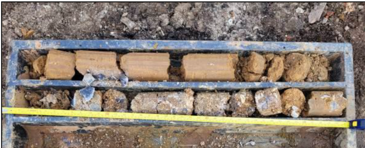
Photograph 1 Removed soil material - BH.01
