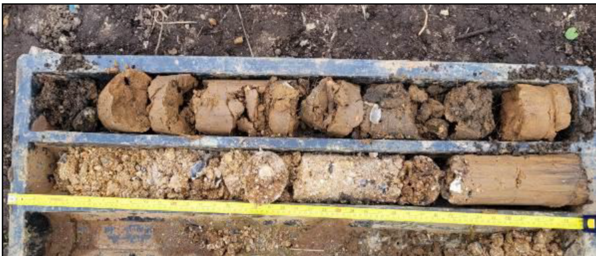
Photograph 5 Removed soil material - BH.05
