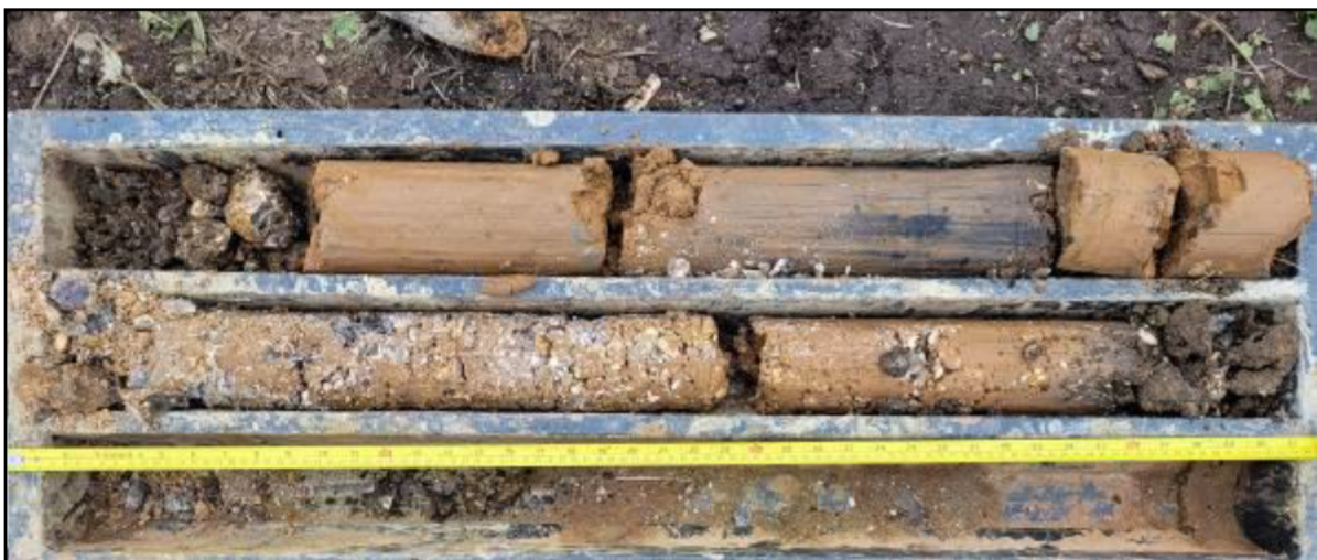
Photograph 6 Removed soil material - BH.06
