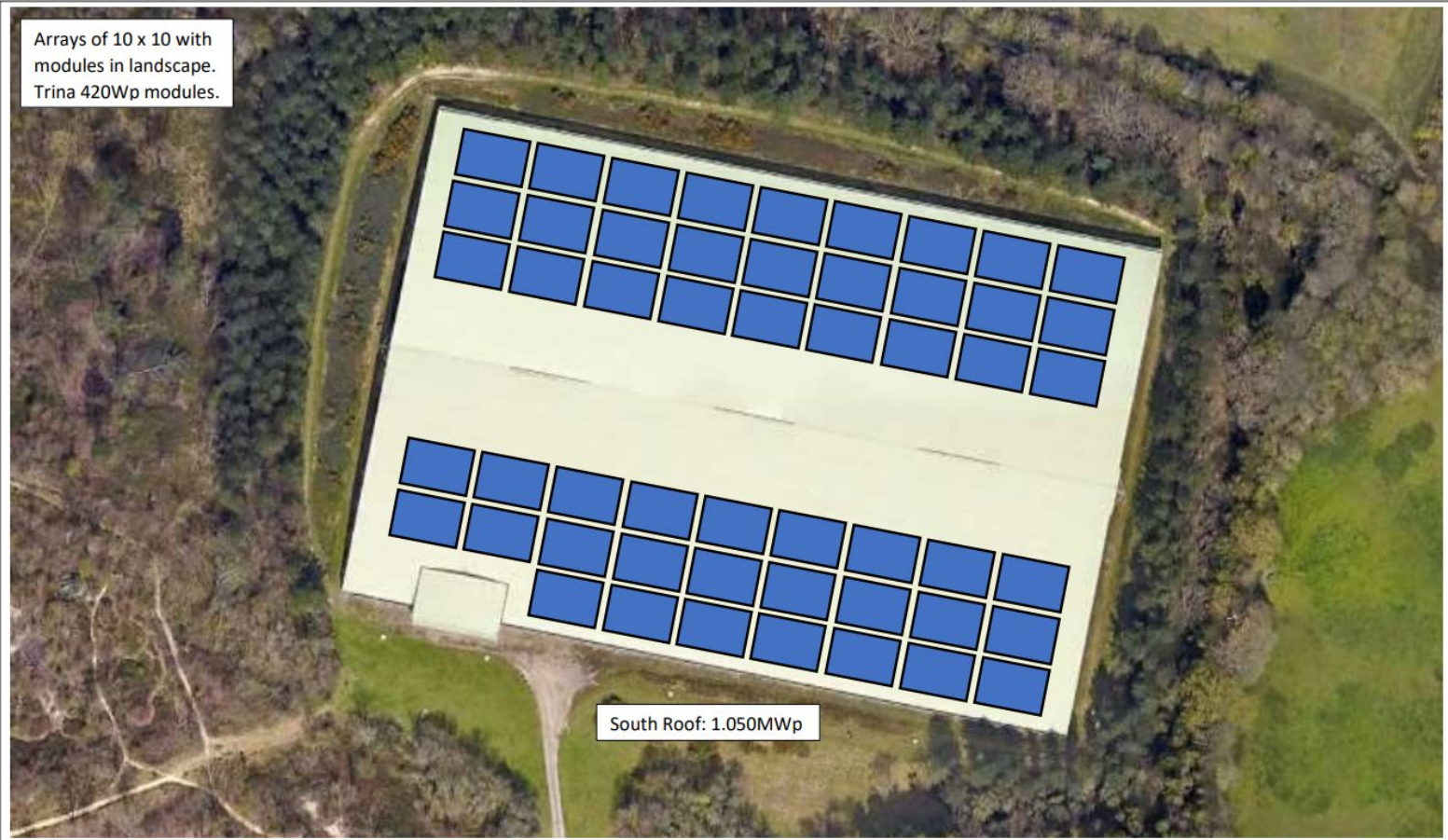
Figure 3. View of the Solar Panels to be installed on the reservoir roof (Portsmouth Water)
