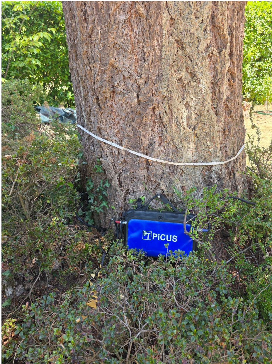
Figure 4. T1 base and tomography equipment at the test level.
