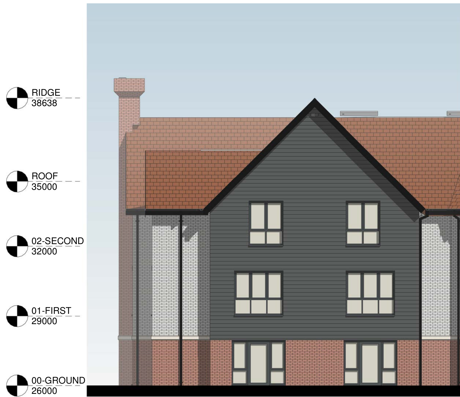
2 North West Elevation 1 : 100
