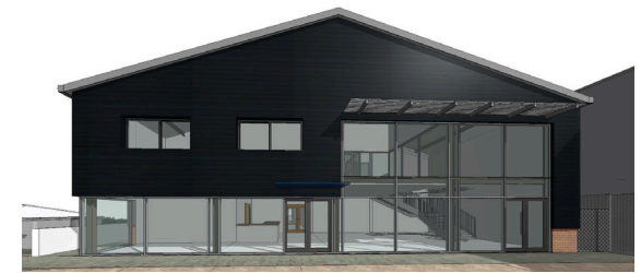
Front elevation with solar shading
