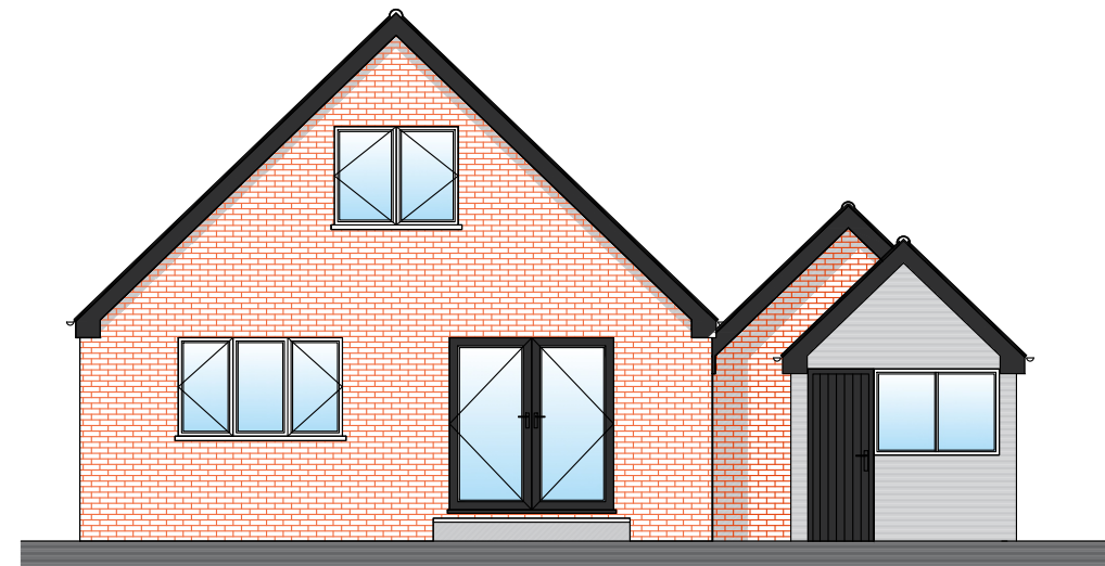
Proposed Rear Elevation 1:100 @ A3
