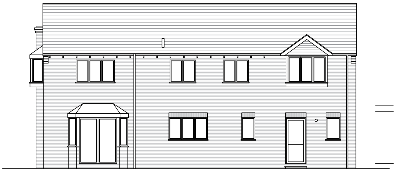
Existing Rear Elevation - 1:100
