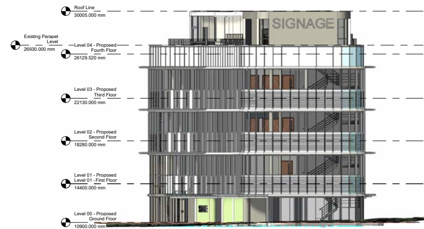
Proposed North Elevation - facing railway station
