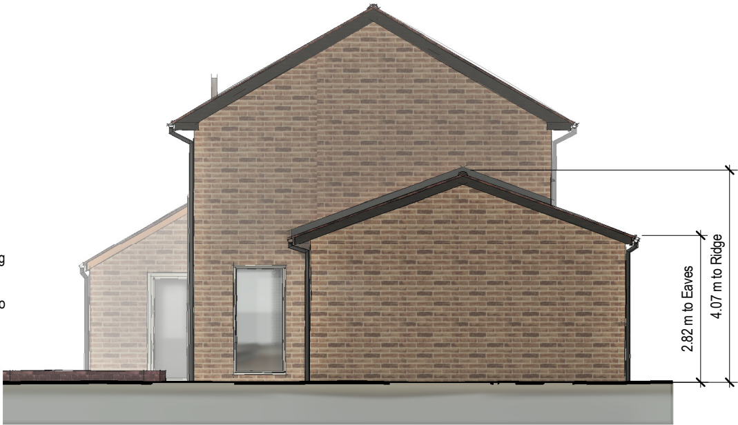
Proposed South Elevation 1 : 100
