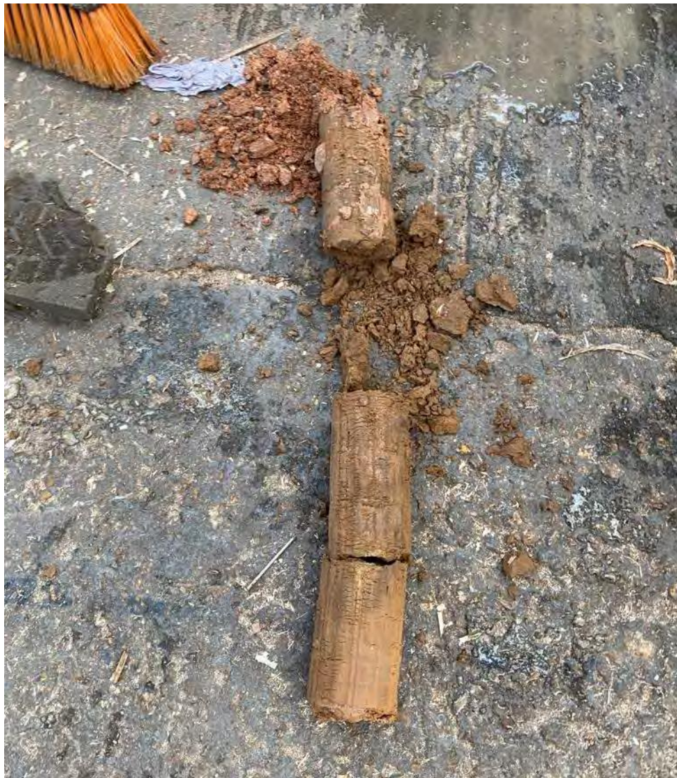
Figure 2 – Typical Natural Soils encountered.
