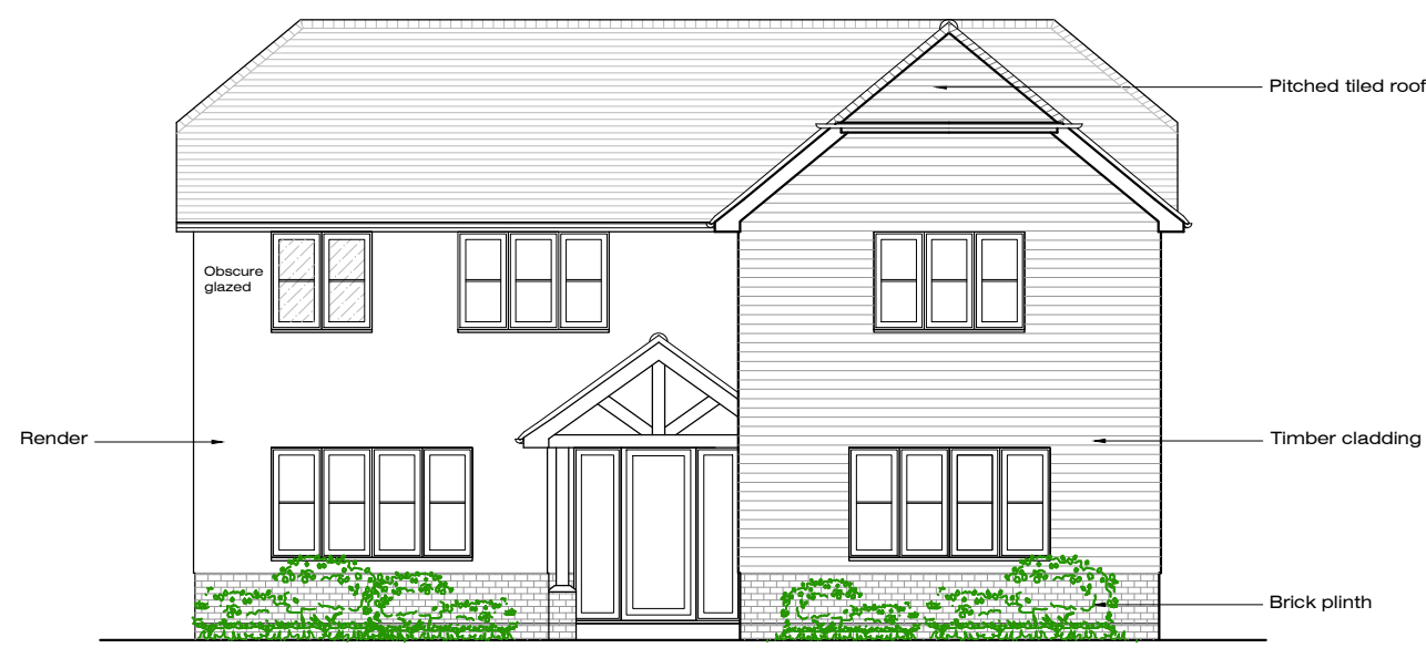
North-East Elevation - As Proposed
