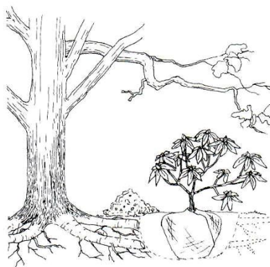
Figure 2: Root severance as a result of planting within RPA Planting Trees and Shrubs. Watson G. W. and Himelick E. B. 1997
