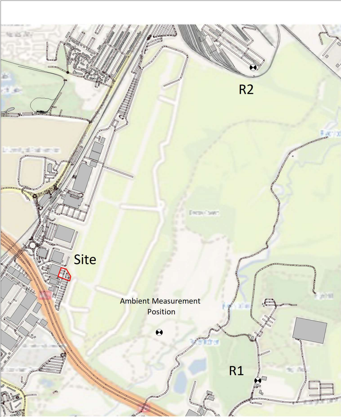
Figure 1 – Site Layout and Noise Measurement Positions
