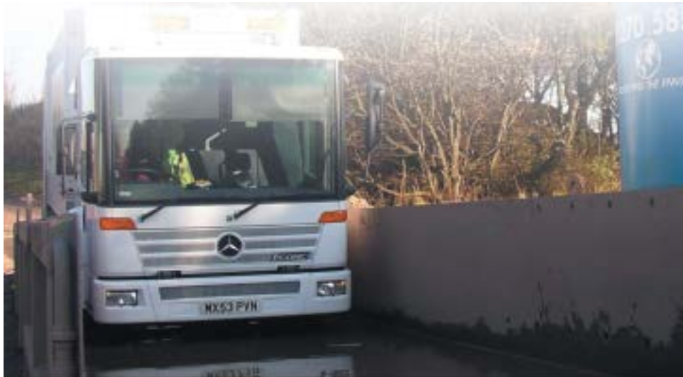
An example of a temporary drive-through bath
