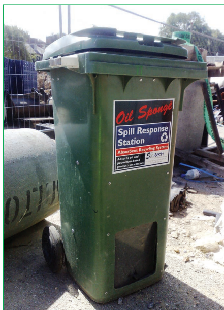
Figure 3.12 Spill response station (courtesy BAM Nuttall)
