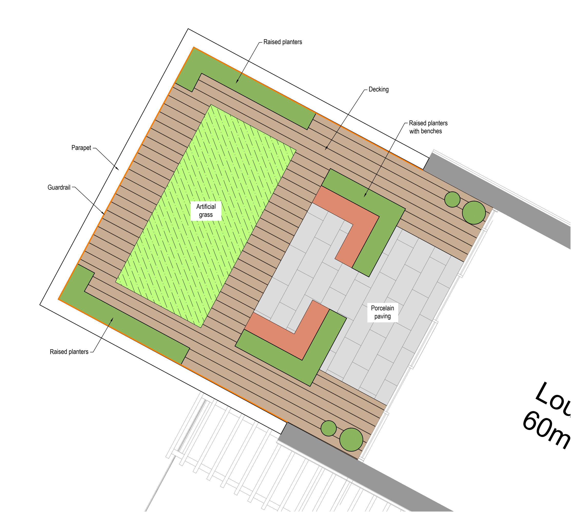
B - Second Floor Terrace
