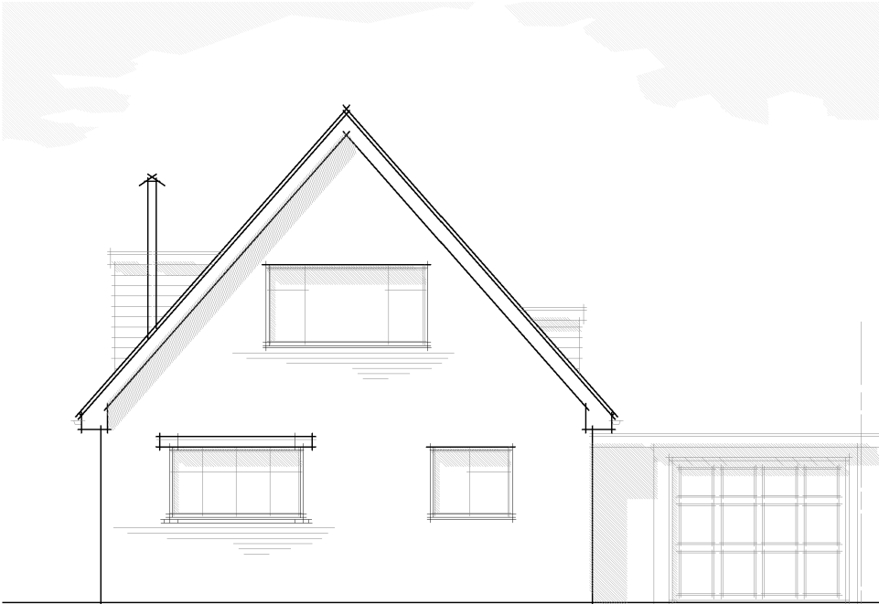
PROPOSED FRONT ELEVATION (facing due east) SCALE 1:100
