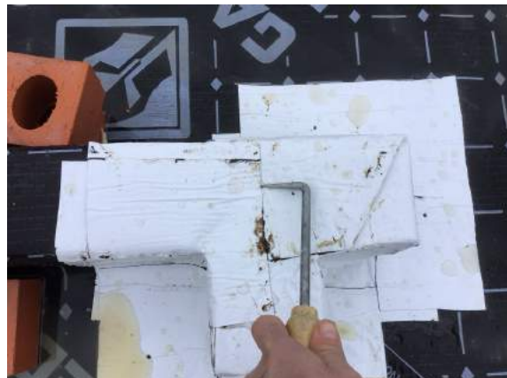
Pick testing all SAGM detailing in plot 67.
