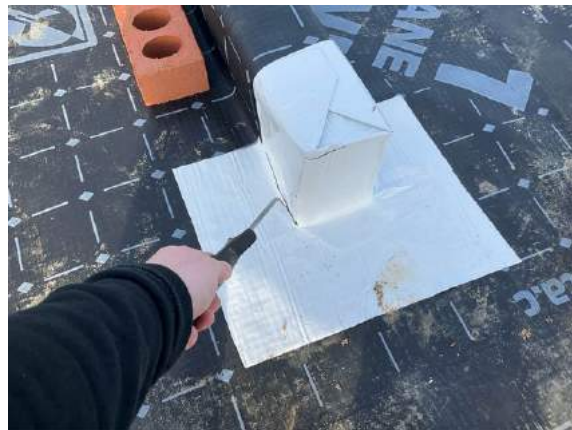
Plot 34. Pick & Probe testing upon sealed corner details.
