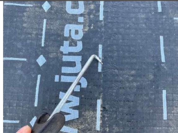
Plot 18. Pick testing along hand welded lap joint.
