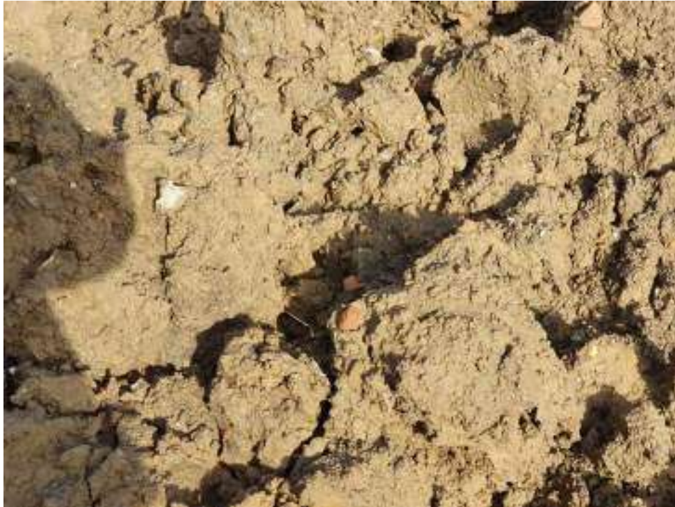
Photograph 3: Sporadic anthropogenic materials within imported Burridge Green subsoil stockpile.
