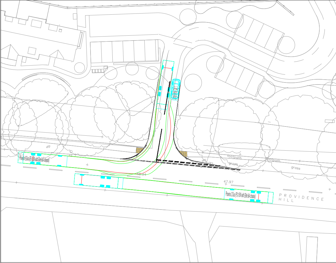
REFUSE VEHICLE TURNING LEFT INTO THE SITE
