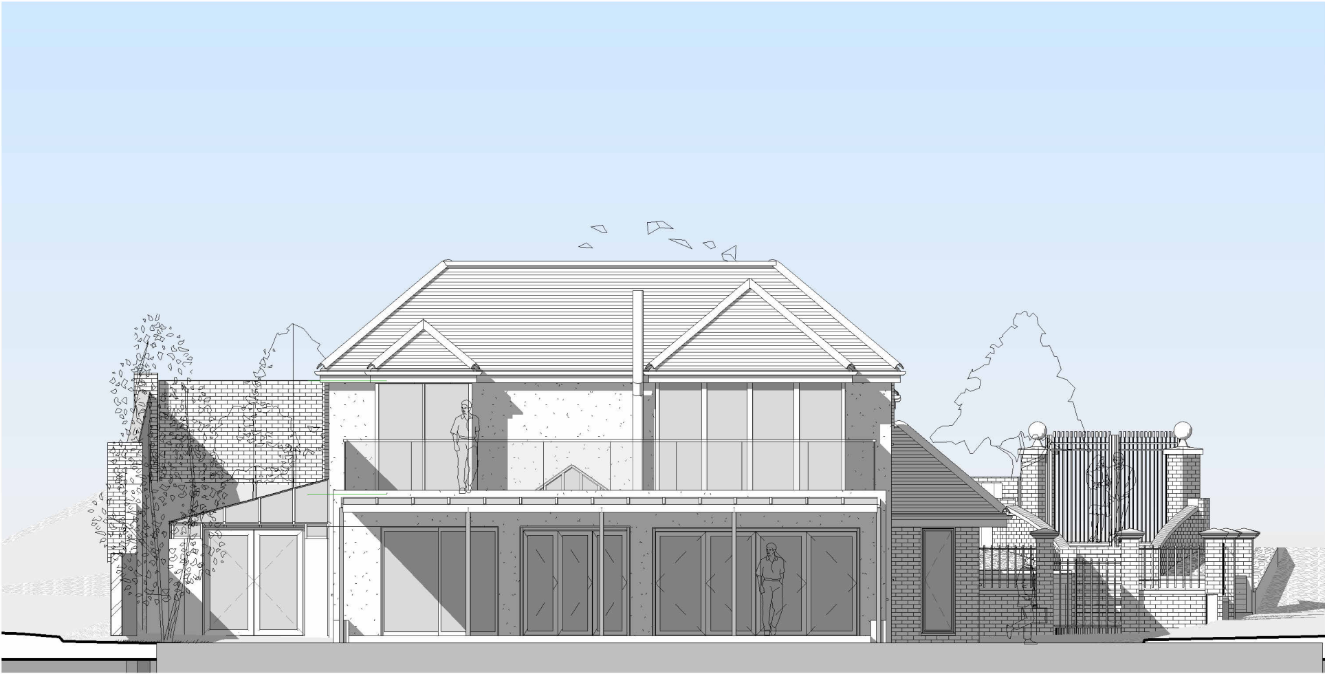
Garden (East) Elevation as Existing 1 : 100
