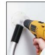
Control measures: shadow vacuuming and using a drill cowl as local extraction
