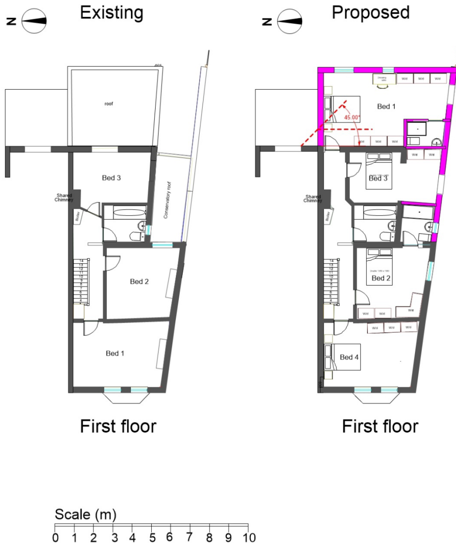
Figure 4. 45 rules diagram overlaid on the first floor plans. The Magenta colour highlights the proposed walls
