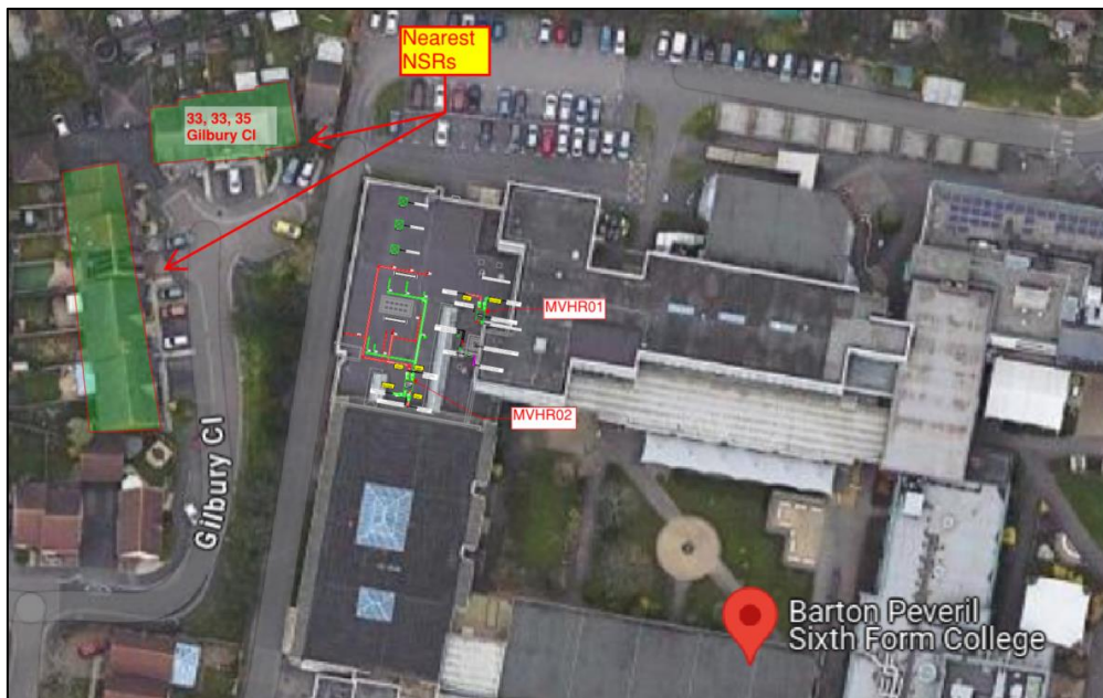
Figure 2-2: Site location plan, roof mounted plant & NSRs
