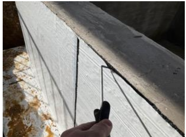
Unit 3/4. Pick test upon termination of Juta GP SAM.
