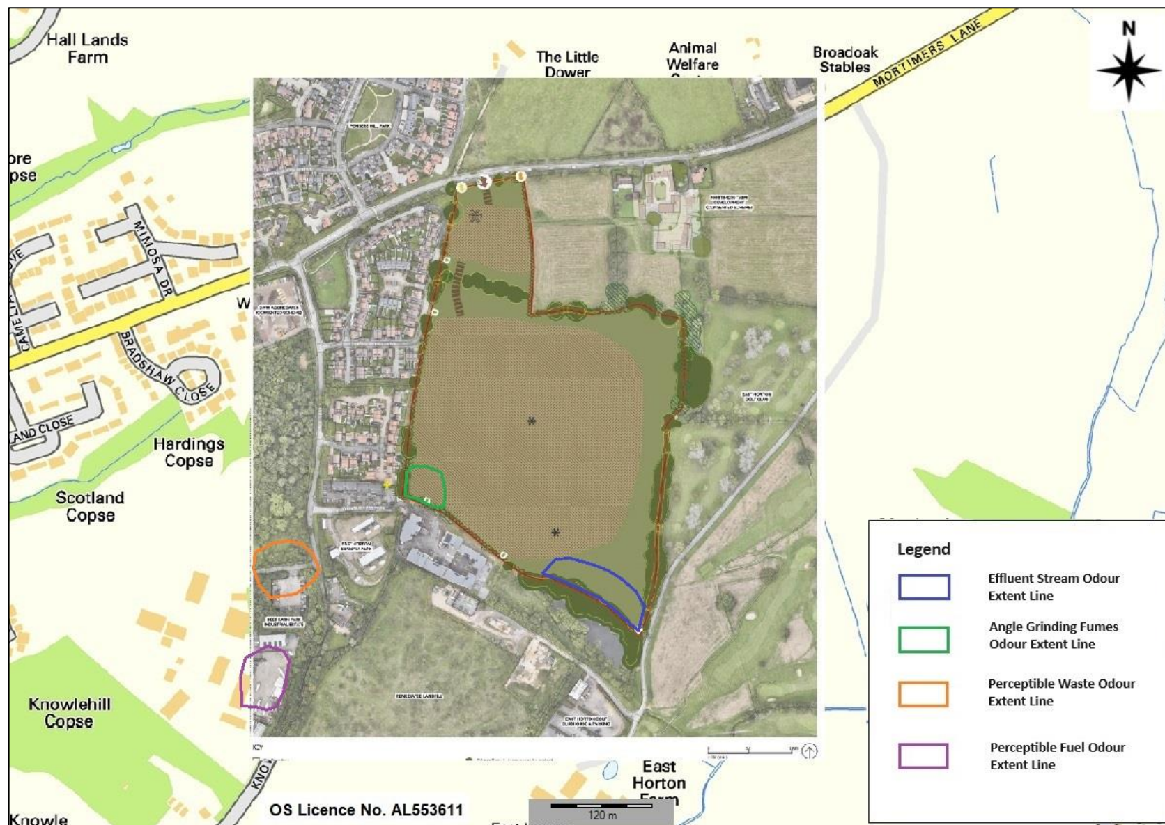
Figure 3-5. Areas of Odour Extent - Survey Observations – 15/02/2024
