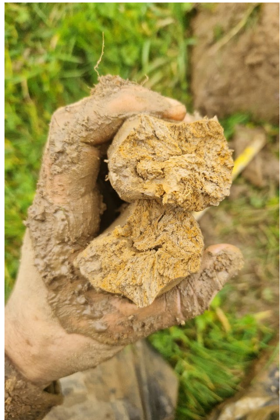
Subsoil mottling observed by auger
