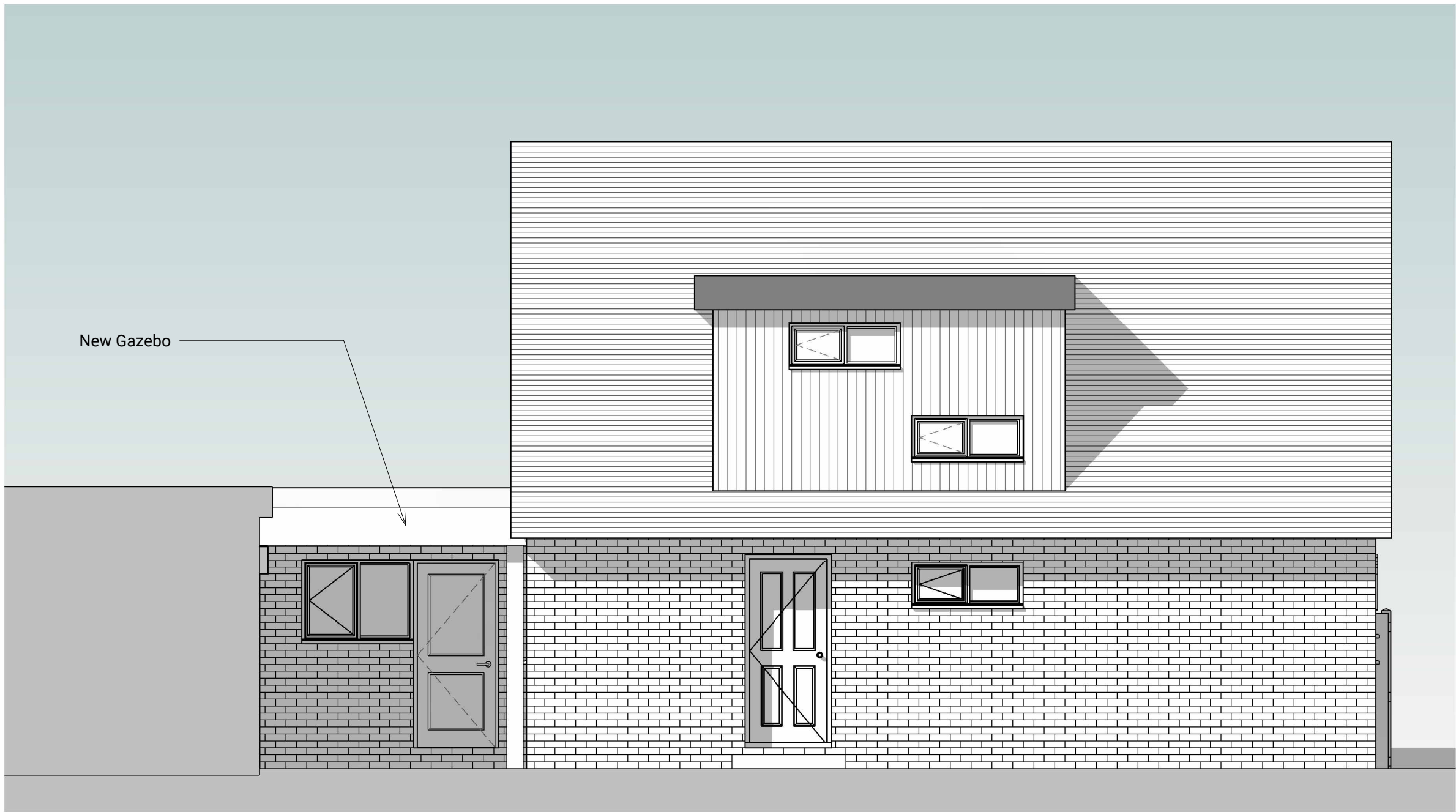
Side Elevation (West) as Proposed 1 : 50
