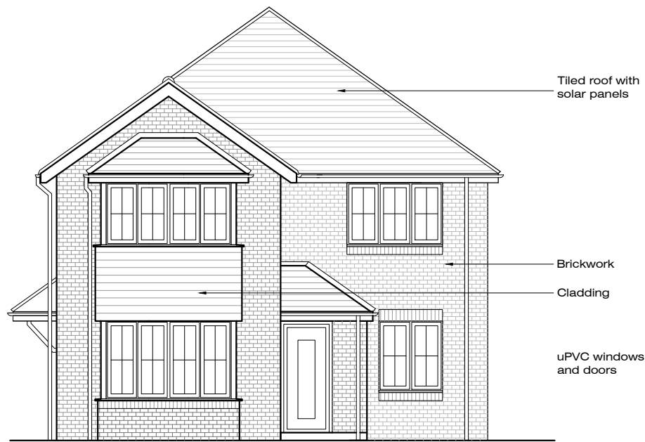
East (Front) Elevation - As Proposed
