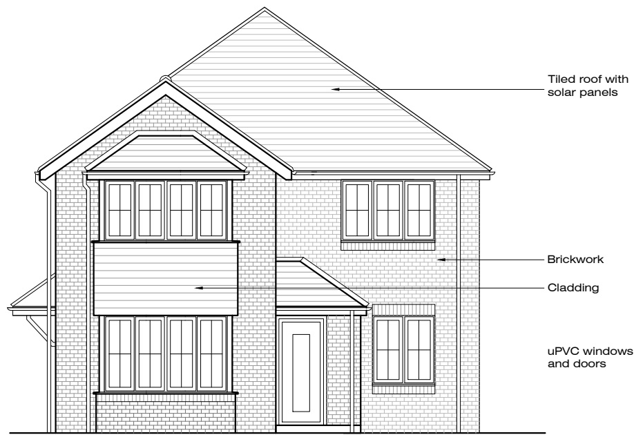
East (Front) Elevation - As Proposed
