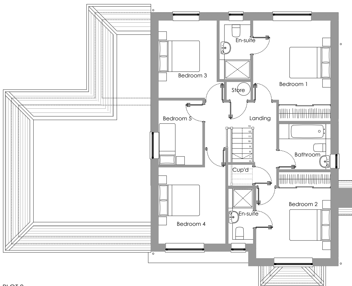
PLOT 9 As Proposed First Floor Plan 1:100
