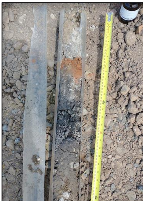
Figure 1 – WS102 core liner showing suspected tarmac material at 0.2mbgl
