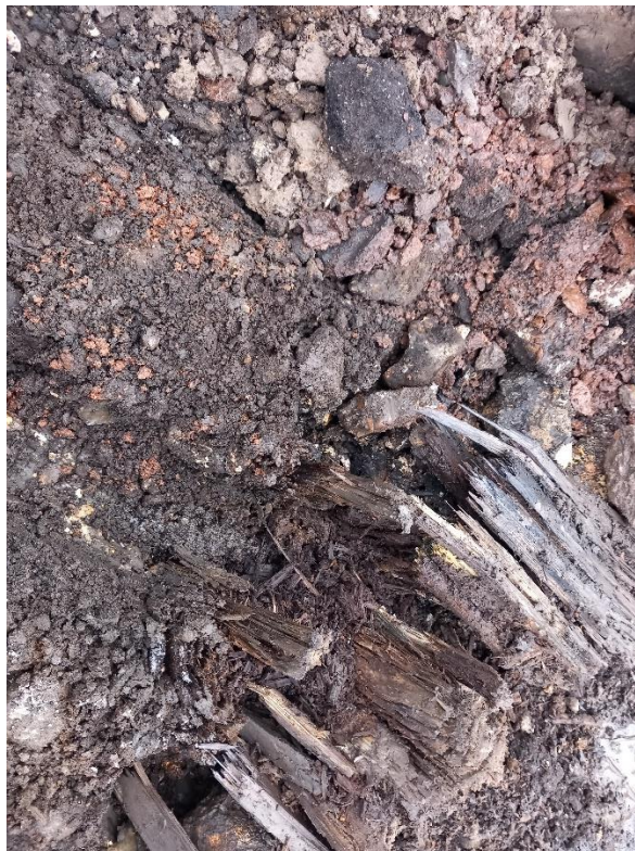
Plate 18: Site Visit 22/12/22 – Wooden sleeper with creosote odour
