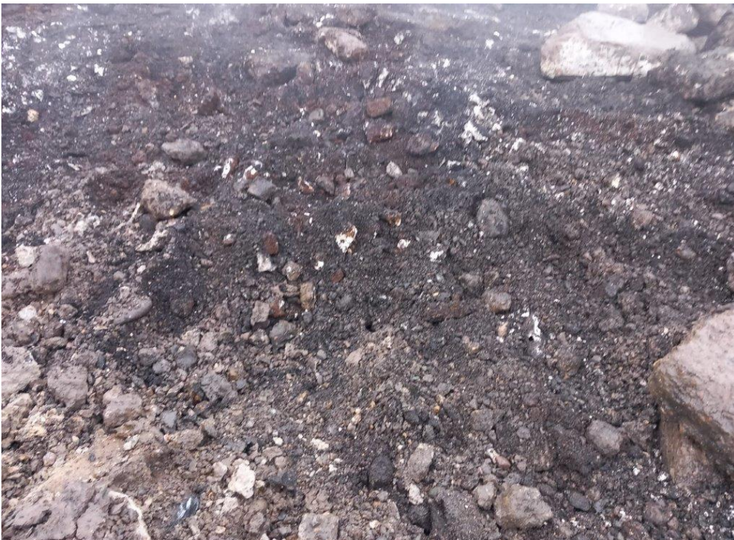
Plate 14: Site Visit 22/12/22 – General granular crush material with silty ash encountered beneath slab in proximity to former rail lines
