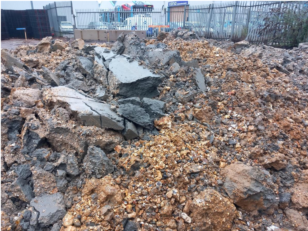
Plate 30: Site Visit 09/03/23 – Stockpiled natural soils of River terrace Deposits and Wittering Formation.
