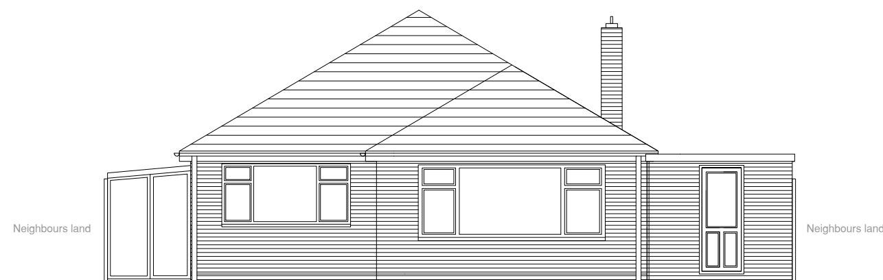
Existing East Rear Elevation
