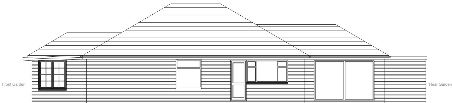
Existing South Side Elevation
