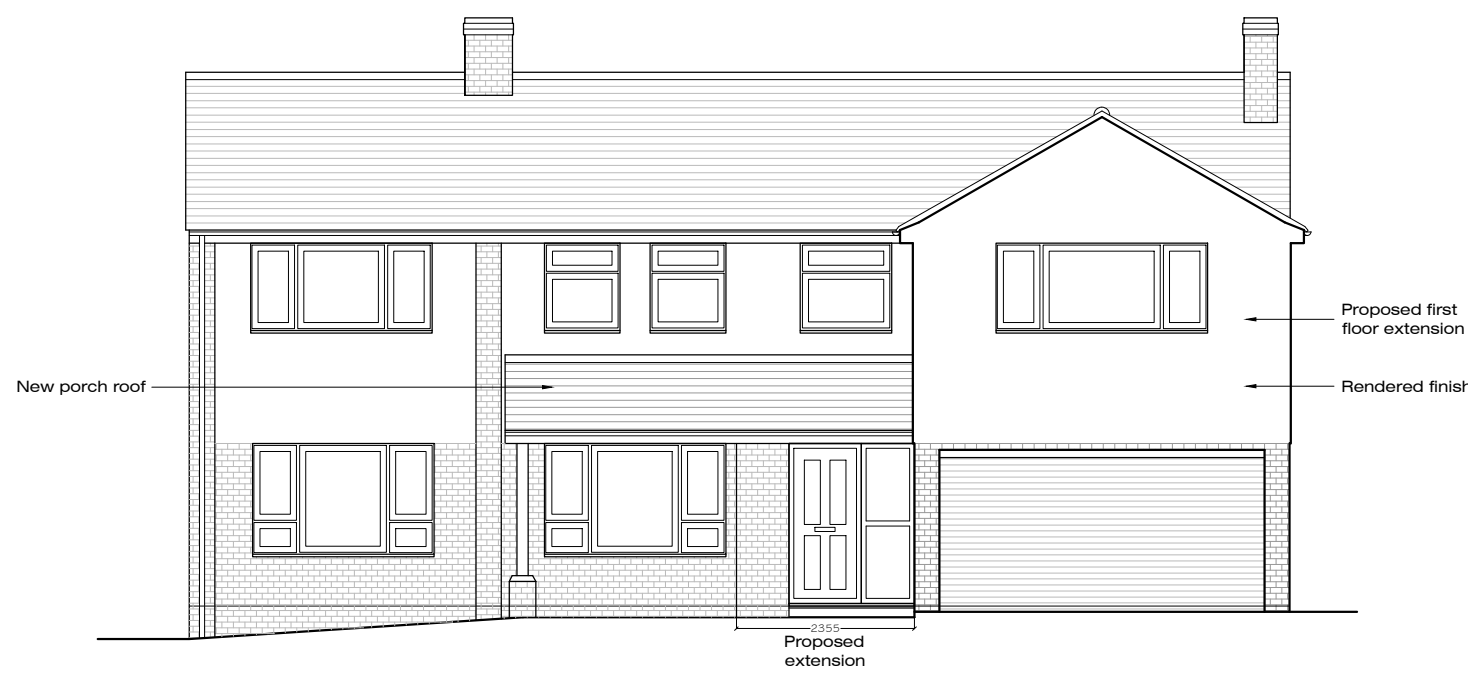
North-East (Front) Elevation - As Proposed 1:100
