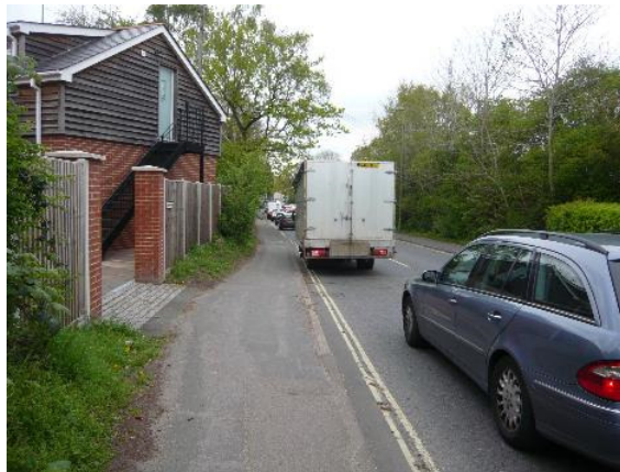
Potentially obstructed visibility to the left and right for a driver exiting an existing property.
