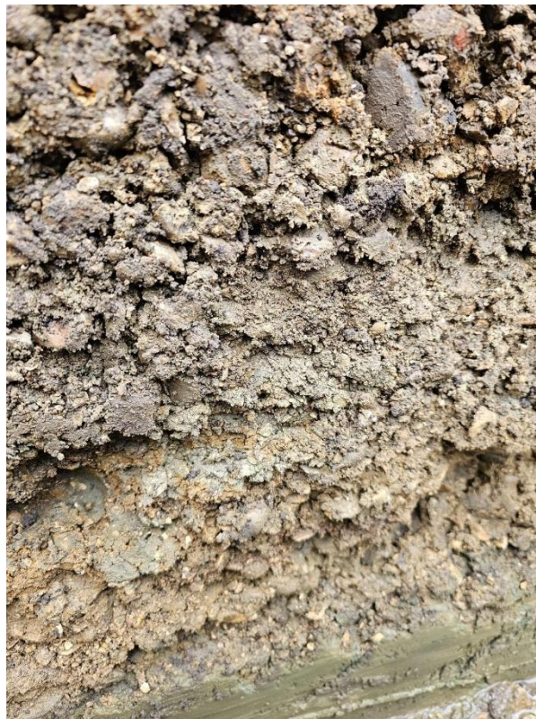
Photograph 5: Observation of site soils consisting of natural clayey sands
