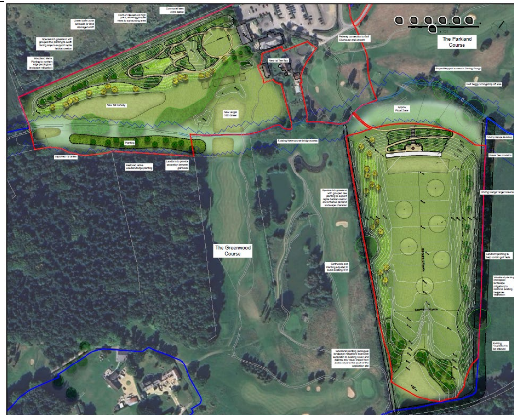
Figure 2 Site plan of the material imported from the donor site to East Horton Golf Club site, including the proposed contours and proposed development across the whole site, created by Deacon Design, February 2025.
