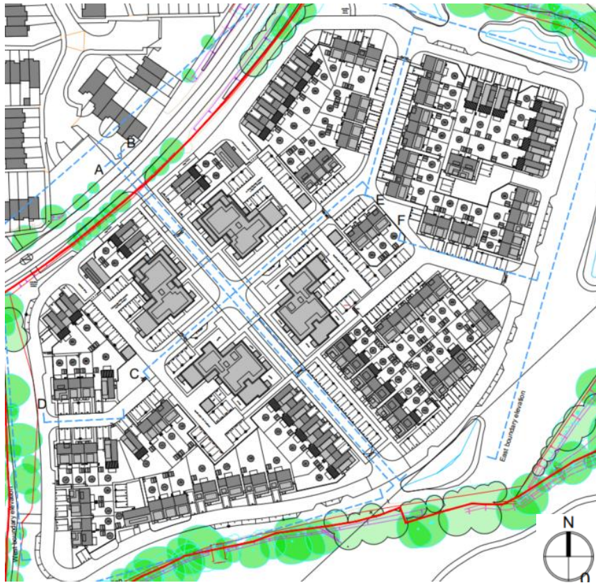
Figure 8 Kings Copse Avenue – Indicative PV roof layout
