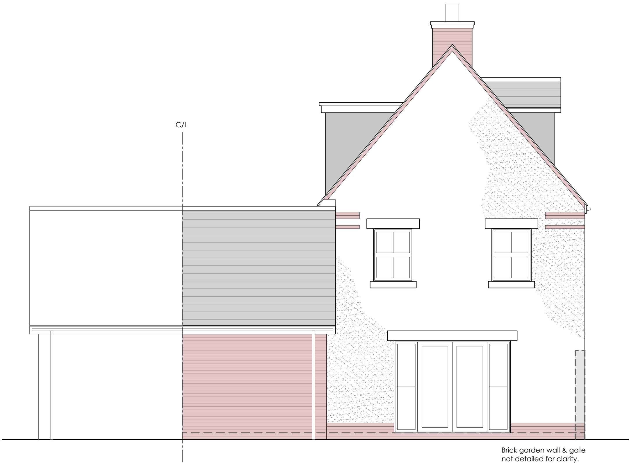
PROPOSED REAR ELEVATION SCALE 1:50 @ A1 / 1:100 @ A3
