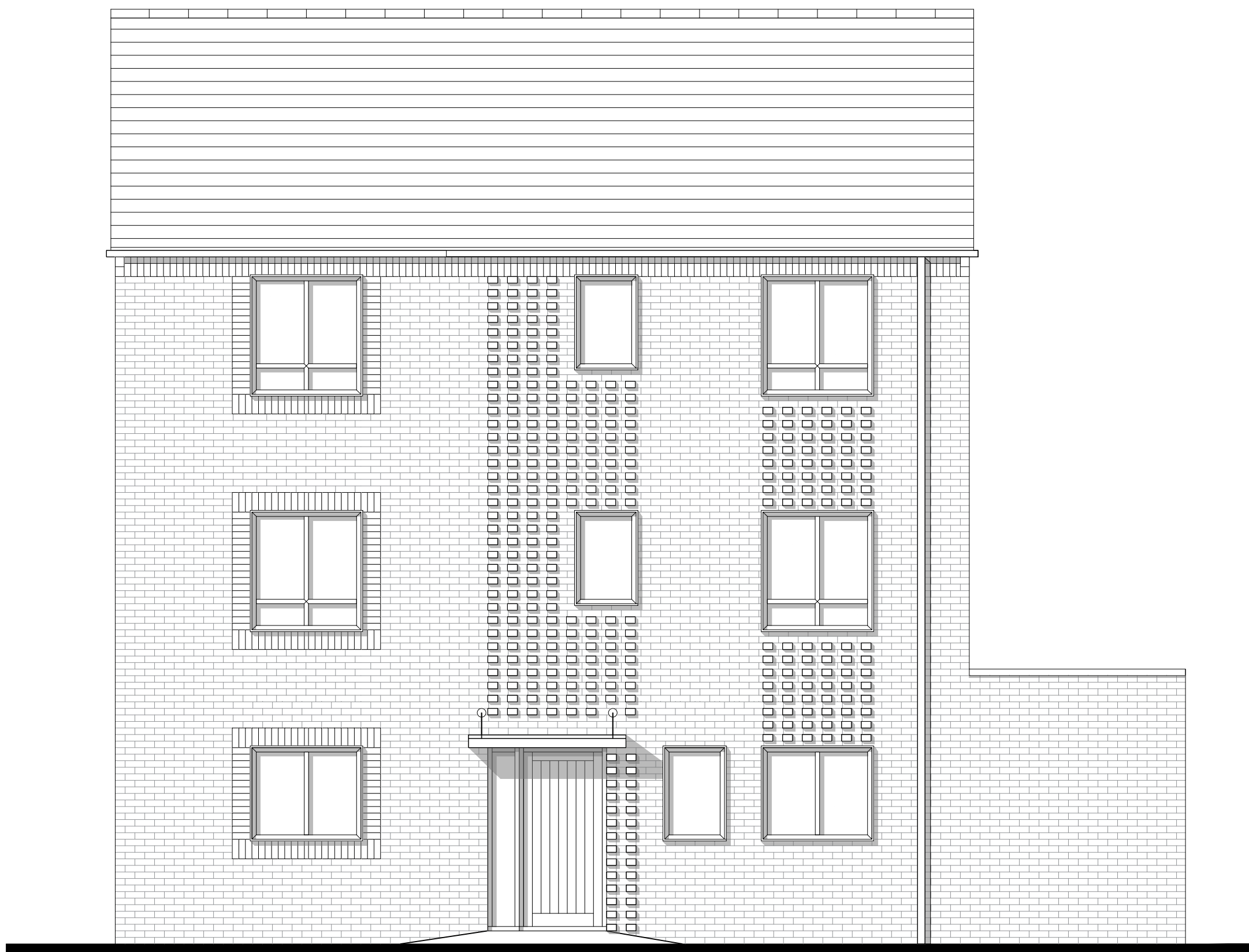
02 Side Elevation No soldier course window surrounds, brick chequers instead, to Plot: 411
