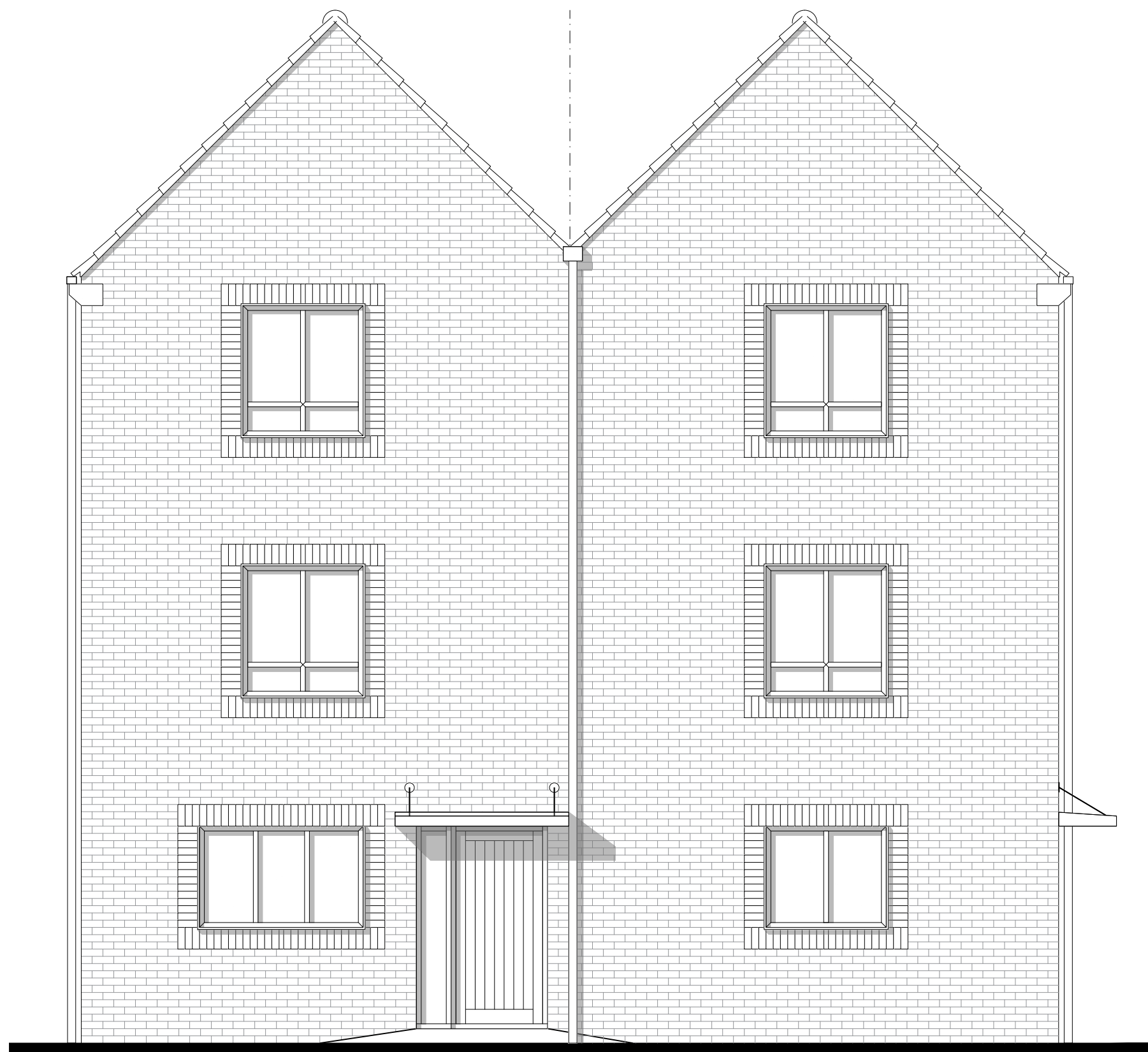
01 Front Elevation No soldier course window surrounds, brick chequers instead, to Plots: 411, 412
