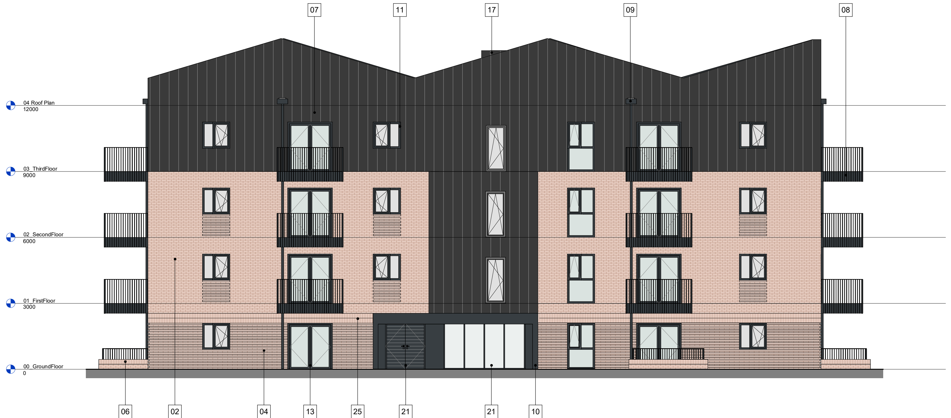
4 Apartment 04 Elevation D
