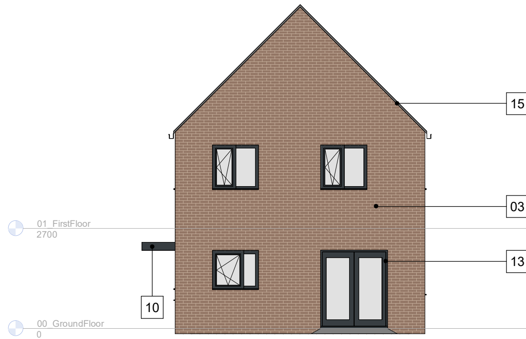
7 Right Side Elevation - House Type JJ
