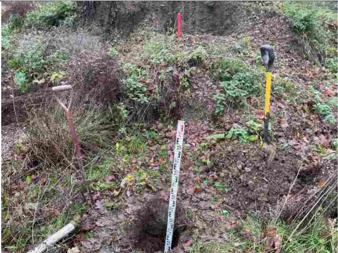
PLATE 9 – New shallow sump dug near original PO2 trial pit
