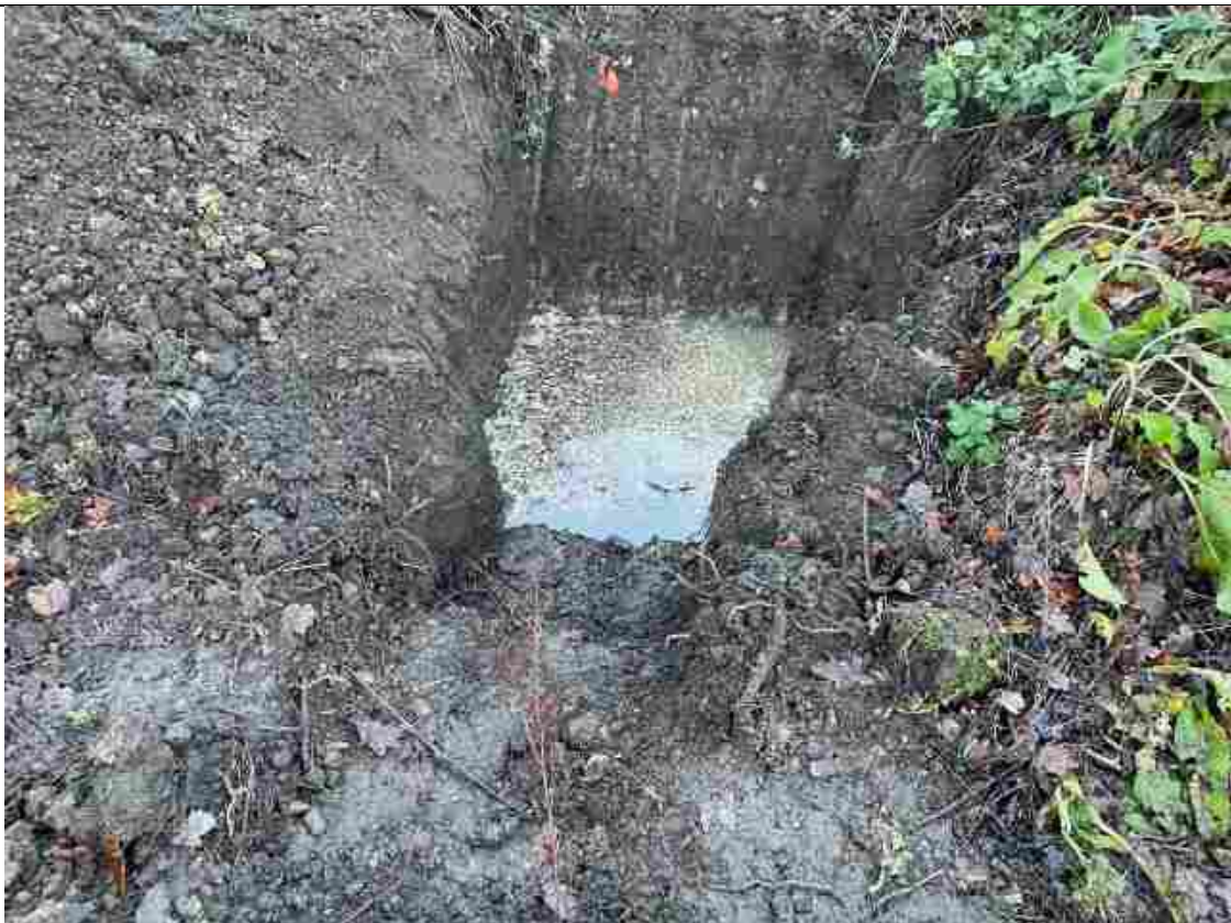
PLATE 5 – Water level in PO1 rose to top of the yellow slightly clayey very gravelly SAND.
