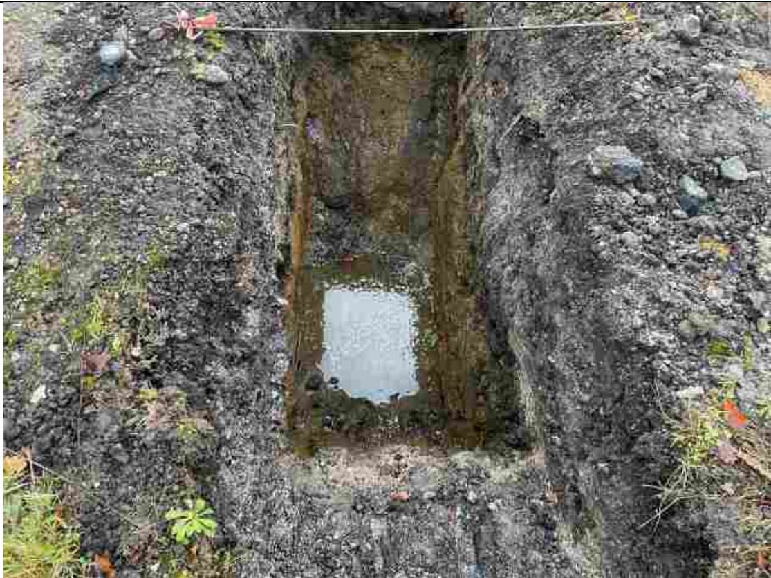
PLATE 17 – Standing water level in Structure 3 trial pit
