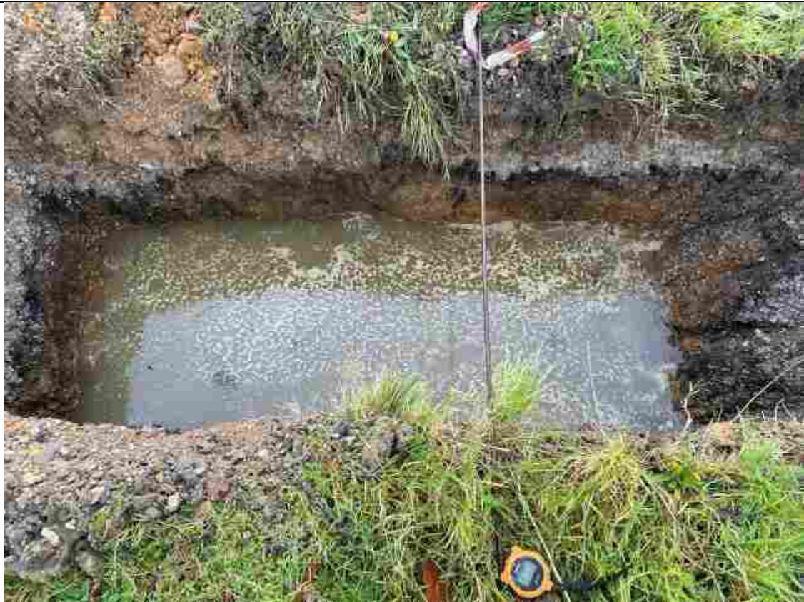
PLATE 19 – Standing water level in Structure 4 trial pit
