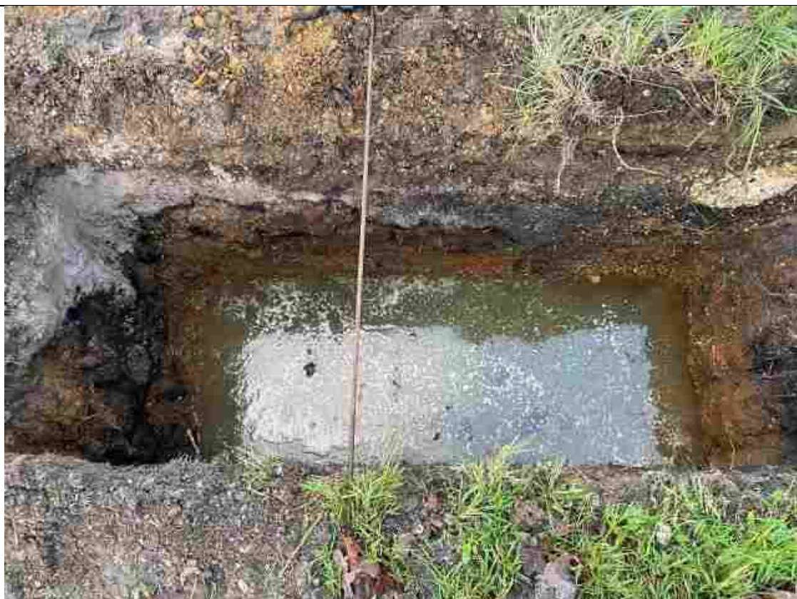
PLATE 15 – Standing water level in Structure 2 trial pit at start of the infiltration test
