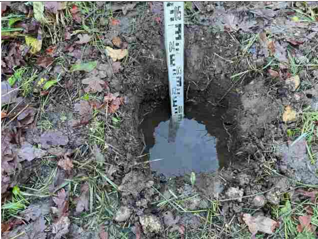
PLATE 11 – PO2 test sump did not drain the pre-commencement 300mm overnight
