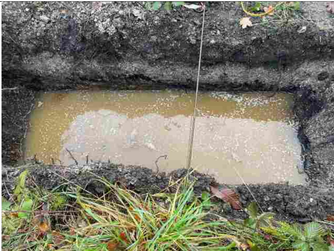
PLATE 13 – Standing water level in Structure 1 trial pit at start of the infiltration test
