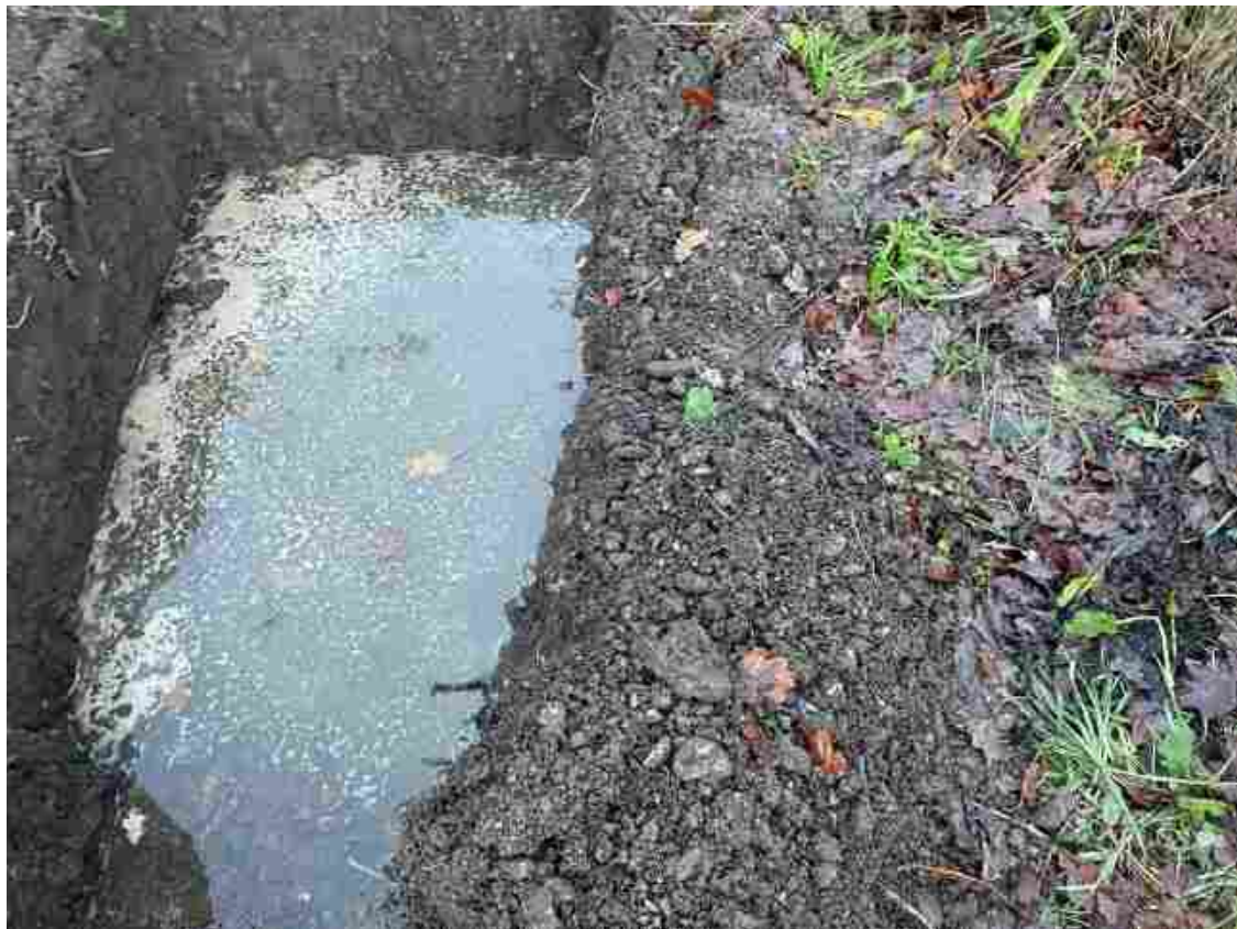
PLATE 8 – Standing water level rose in PO2 trial pit
