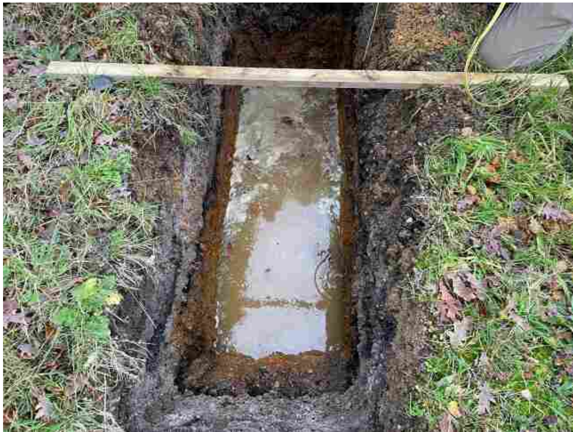
PLATE 20 – Structure 5 trial pit an hour after being dug
