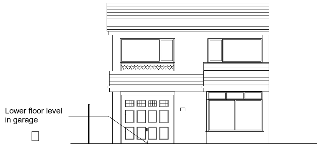
EXISTING SOUTH WEST ELEVATION
